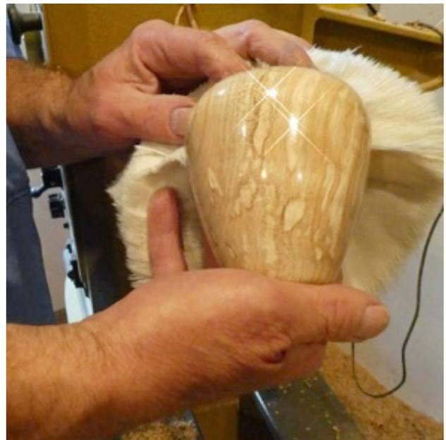
*Run the buffing wheel at about 1000 RPM. Hold the piece securely.*
