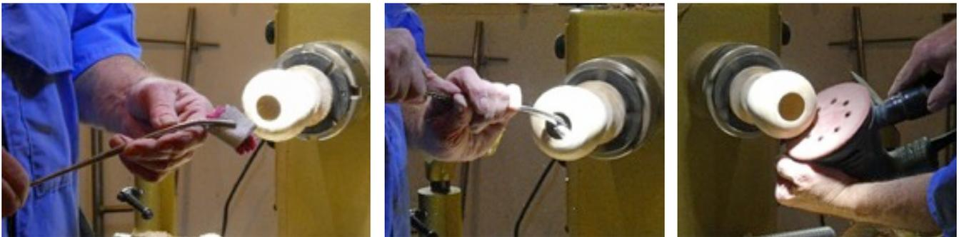
*Sand the inside using a hemostat clamping sandpaper around a wad of cloth. Move the angle of the sandpaper to match the angle of the inside contour. Sand the outside with a random orbit sander hooked up to a vacuum.*
